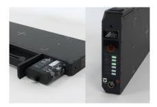
The battery can be changed quickly and easily. LEDs indicate the status of the connection type, battery and sensor.
